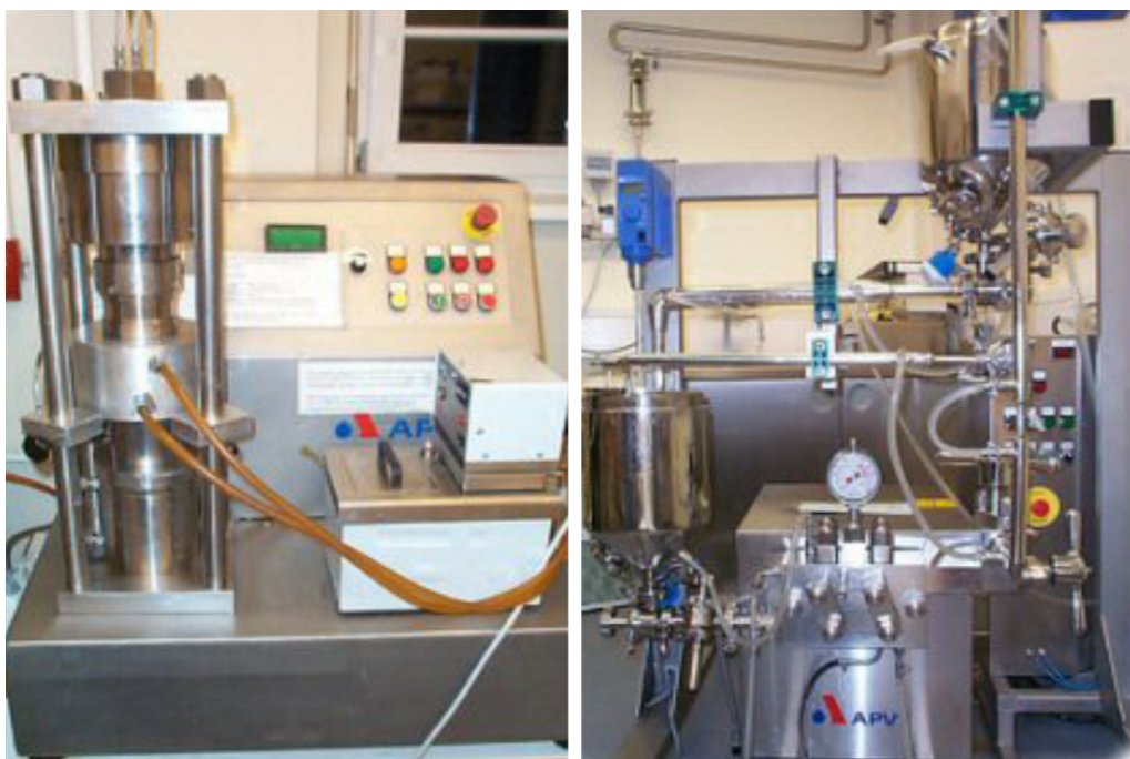
Fig. 2. APV Micron LAB 40 for lab scale production unit used for 40 mL batch (left) and LAB 60 for 10 kg batch production (right).
