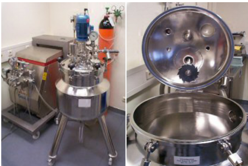
Fig. 3. APV Gaulin C 5.5 high pressure homogenizer with capacity: 150L/h (left) and 60 kg supply/product container (right) with open lid showing the dissolver disk for preparing the pre-emulsion.
